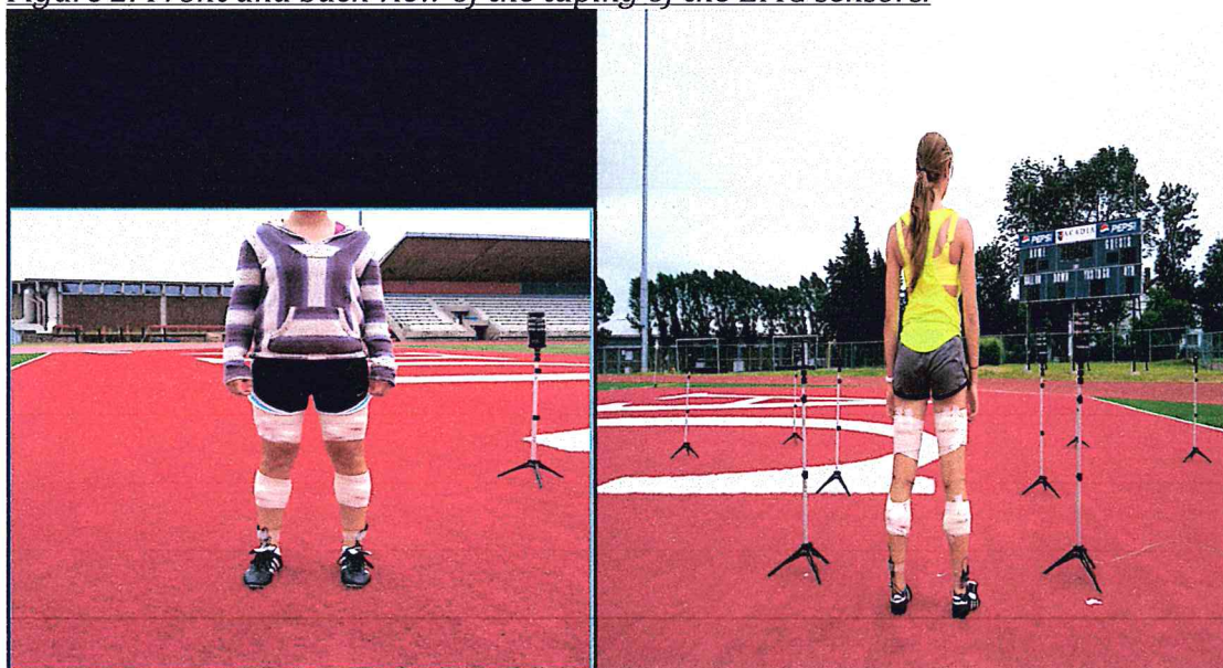
Figure 2: Front and back view of the taping of the EMG sensors.
