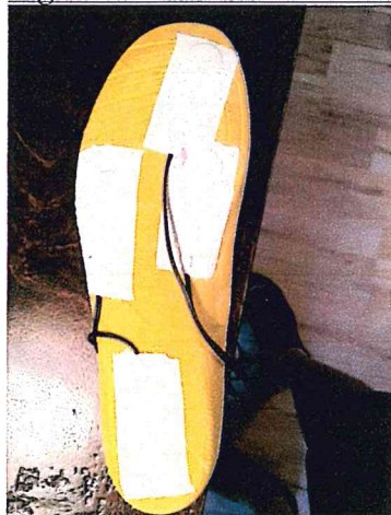
Figure 5: Foot Switch Placements
