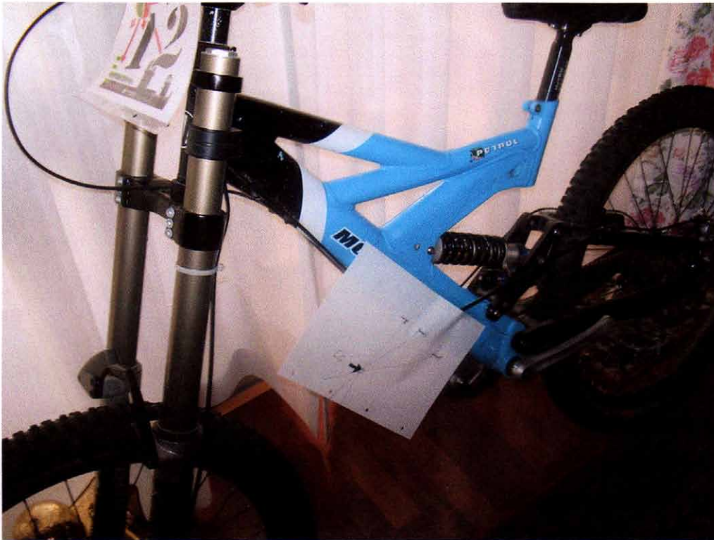
Finding the centre of mass of the bicycle by hanging it from 3 points and drawing lines.
