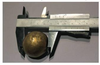
A vernier calliper has sliding jaws which are moved so they touch both sides of the ball.
