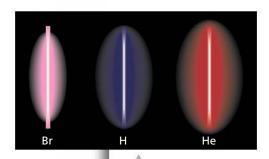
**Figure 7.4** Discharge tubes containing bromine, hydrogen and helium.
