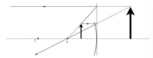
In Figure 11.41 the ray doesn't actually originate from F but appears to come from that direction. This is how you would see the image of your face when looking into a shaving/make up mirror.
