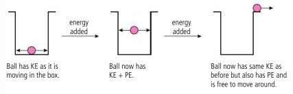
**Figure 3.29** A ball-in-a-box model of change of state.
