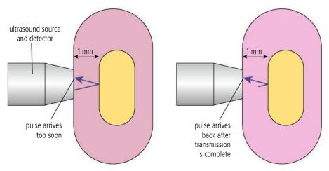
As the speed of sound in the body is approximately 1500 m s<sup>-1</sup>, the time taken to travel 2 mm is  $1.3 \times 10^{-6}$  s so the duration of the pulse should be no longer than this. To be able to use the signal there must be at least one complete cycle of the wave so in this case the wavelength should be less than 2 mm which is equivalent to a minimum frequency of 750 kHz ( $f = \frac{v}{\lambda}$ ).
