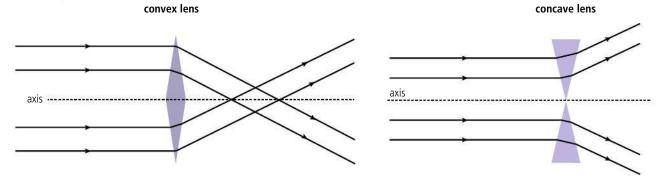
**Figure 11.2** Refraction through lenses.
