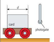
**Figure 2.9** A card and photogate used to measure instantaneous velocity.
