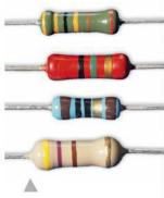
A resistor is a component with a known resistance. You can work out the resistance from the colours.
