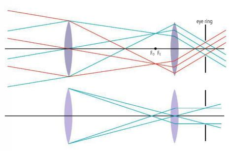
**Figure 11.62** The eye ring is the image of the objective in the eyepiece.
