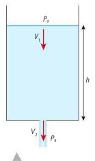
**Figure 10.79** Water running out of a hole in a bucket.
