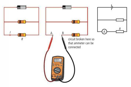
**Figure 6.51** The ammeter is connected to measure the current through *R*.
