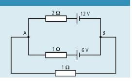
**50** Find the current and pd measured by the meters in Figure 6.64.
