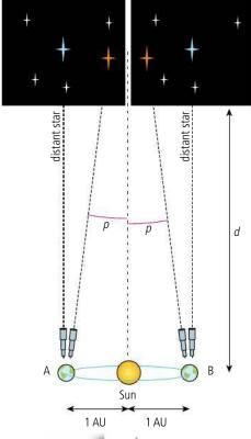
**Figure 12.4** Measuring the distance to a star.
