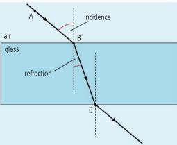
path of the ray. If you don't have a light source you can use an alternative method with pins. Place two pins on one side of the block in positions A and B then, looking through the block, place a third pin in line with the other two. Joining the dots will give the path of a ray from A through the block.
