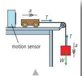
**Figure 2.76** Apparatus for finding the relationship between force and acceleration.
