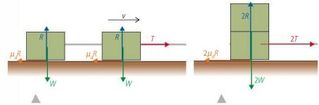
Figure 2.56 Two blocks joined with a rope.
