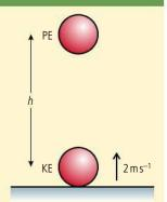
**Figure 2.110** Work is done lifting the ball so it gains PE.
