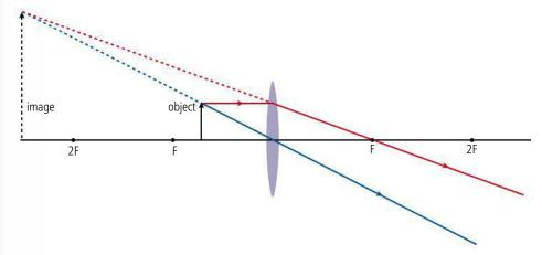
When the object is closer than F (Figure 11.15) the object is so close to the lens that the lens cannot bend the rays enough to bring them together.
