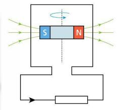
A generator as covered in chapter 6 consists of a rotating coil in a magnetic field. As the flux enclosed by the coil changes, an emf is induced that causes an alternating current to flow in an external circuit. The rotating coil is connected to the stationary circuit using slip rings and a sliding contact. This contact will wear out after time so an alternative solution is to use stationary coils and moving magnets, as in Figure 8.7.
