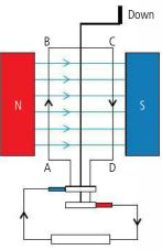
When a generator is connected to a load the direction of current in the coils opposes the change producing it. To slow down an electric car the rotating coil of the motor is used as a generator to charge the battery: this provides effective braking and saves energy.
