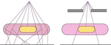
Another way of reducing scatter is to introduce a grid between the object and photo-plate as in Figure 11.81. This only allows rays that pass through the sample in a straight line from the source to arrive at the photo-plate.
