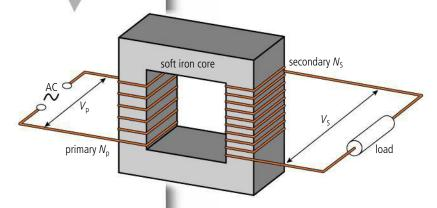
A transformer consists of two coils wound on a common soft iron core as shown in Figure 6.111. The primary coil is connected to an AC supply. This causes a changing magnetic field inside the coil. This field is made stronger by the presence of the soft iron core which itself becomes magnetic (temporarily). Since the secondary is wound around the same former, it will have a changing magnetic field within it, which induces an emf in its coils.
