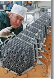
Pellets of nuclear fuel are stacked into tubes that are bundled together before being put into the reactor.
