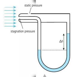
**Figure 10.83** Measuring the speed of an airplane.
