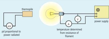
Figure 8.30 shows the results from this experiment. The pd measured across the thermopile is on the y-axis and the filament temperature on the x-axis.
