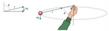
For the motion to be horizontal there will be no vertical acceleration so the weight must be balanced by the vertical component of tension ( $T \cos \theta = mg$ ). This means that the string cannot be horizontal but will always be at an angle as shown in Figure 4.7. The centripetal force is provided by the horizontal component of tension ( $T \sin \theta = \frac{mv^2}{r}$ ), which is equal to the vector sum of the two forces.
