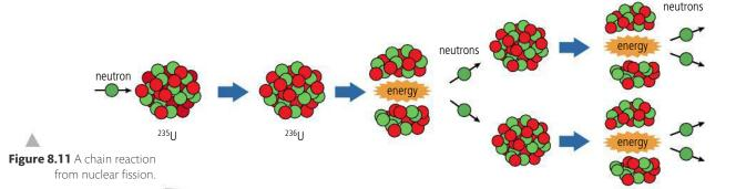
Using the word moderation sounds like the moderator slows down the reaction, but it doesn't. The moderator slows down the neutrons, enabling the chain reaction. If the moderator was removed the reaction would slow down.
