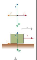
**Figure 2.55** The force experienced by a block pulled along a table.
