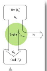
**Figure 10.56** Energy flow for a heat engine.
