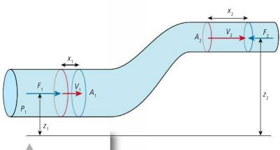
**Figure 10.78** Water flowing uphill in a narrowing pipe.
