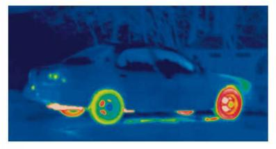
This thermogram of a car shows how the wheels have become hot owing to friction between the road and the tyres, and the brakes pads and discs.
