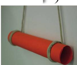
**Figure 10.87** The falling cylinder is made to spin as the string unwinds.
