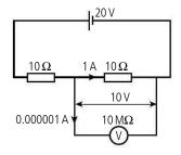
If the same meter is used to measure the pd across a  $10\,\mathrm{M}\Omega$  resistor (Figure 6.50), half of the current is diverted around the component resulting in a lower potential difference.
