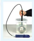
A pressure sensor can also be used in an experiment to show the relationship between pressure and temperature. This time a flask of fixed volume is placed in a water bath as shown in the photo and Figure 3.48. A temperature sensor measures the temperature of the gas while a pressure sensor measures its pressure. The temperature of the gas is changed by heating the water, and the pressure and temperature are recorded simultaneously.
