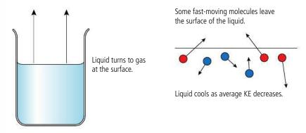
**Figure 3.30** A microscopic model of evaporation.
