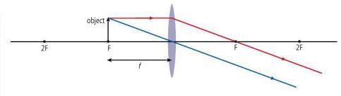
When the object is at F (Figure 11.14) there doesn't seem to be an image since the rays do not cross over. However, if viewed from the right hand side the rays appear to come from a very distant point. We can say that the image is virtual and at an infinite distance to the left of the lens. You could also argue that there was a real image an infinite distance to the right but that image cannot be viewed.
