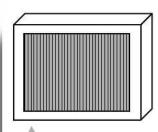
**Figure 5.105** Diffraction grating (the number of lines per millimetre can be very high: school versions usually have 600 lines per millimetre).
