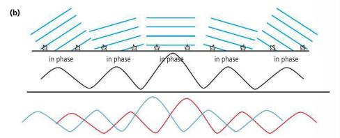
An image of the stars can be built up from the interference pattern data by a process known as *aperture synthesis*. The resulting increase in resolving power is equivalent to building one huge telescope with diameter equal to the separation of the telescopes. Using this technique, telescopes can be as wide as the Earth itself.
