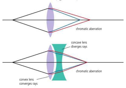
**Figure 11.32** Chromatic aberration and an achromatic doublet. The deviation of rays in the diagram is exaggerated to show what is happening.
