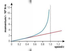
Figure 9.52 Momentum calculated for different velocities using the classical (red) and relativistic (blue) formulae.
