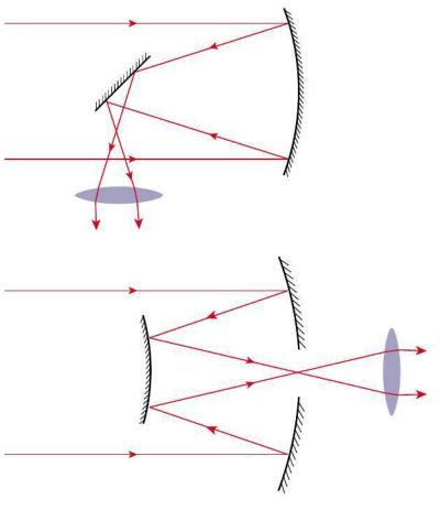
In these telescopes the eyepiece lens can be omitted and a CCD (*charge coupled device*) placed at the focal point of the mirrors. This is the light sensitive part of a digital camera and can be used to produce a digital image of the stars which can be processed by a computer to produce an image or to do spectral analysis on the light from different objects.
