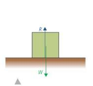
Figure 2.51 A free body diagram of a box resting on the ground.
