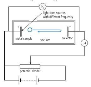
Light from a source of known frequency passes into the apparatus through a small window. If the photons have enough energy, electrons will be emitted from the metal sample. Some of these electrons travel across the tube to the collector causing a current to flow in the circuit; this current is measured by the microammeter. The potential divider is now adjusted until none of the electrons reach the collector (as in
