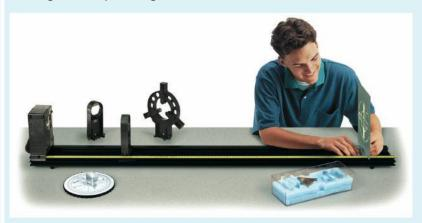
To measure the focal length of a concave lens is not so straightforward since the image is virtual. However, if a virtual image is used then a real image can be projected onto a screen. Figure 11.30 shows how this can be done.
