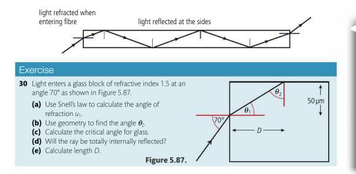
**Figure 5.86** Light reflected along a fibre.
