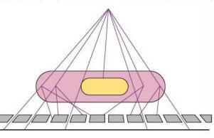
**Figure 11.80** Comparing scatter from wide beam and narrow beam.
