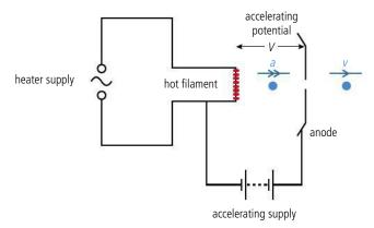
The filament, made hot by an AC supply, liberates electrons which are accelerated towards the anode by the accelerating pd. Electrons travelling in the direction of the hole in the anode pass through and continue with constant velocity.
