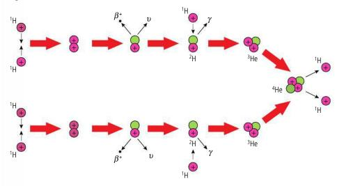
Figure 12.13 The protonproton cycle.
