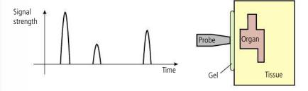
The thickness of the organ can be found from the time between the pulses. Note that due to attenuation the second pulse is smaller than the first but the third pulse is larger since there is a big impedance difference between tissue and air so the percentage reflection is high.
