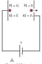
**Figure 9.53** Accelerating a proton.
