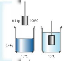
**Figure 3.34** Measuring the specific heat capacity of a metal.
