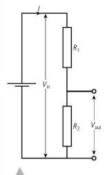
**Figure 6.65** potential divider circuit consists of two series resistors.
