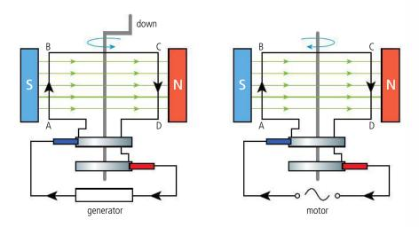
**Figure 8.22** When the coil is turned current flows, but if a battery makes current flow then the coil turns in the opposite direction (note AC so direction of current changes every half revolution).
