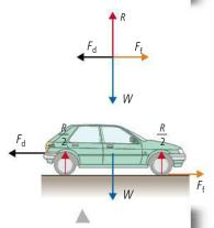
**Figure 2.113** The forces acting on a car travelling at constant velocity.
