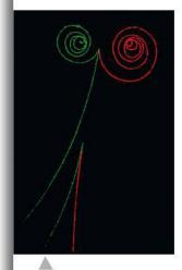
Electrons (green) and positrons (red) are formed from gamma photons. Notice how the *B* field (into page) causes them to curve in opposite directions. The bottom pair has more KE than the top pair, so the radius of their path is greater.
