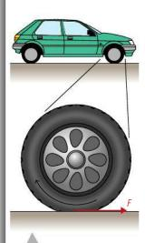
**Figure 2.60** Friction pushes the car forwards.
