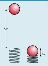
**Figure 2.112** In this example the spring is compressed, not stretched, but Hooke's law still applies.
