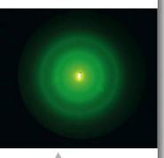
Diffraction of electrons by a graphite film.
