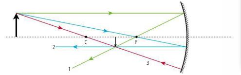
**Figure 11.33** Parallel rays reflecting off a concave mirror.
