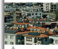
Solar heating panels on top of houses in Antalya. The position of solar panels depends on the amount and direction of sunlight as well as the design of the building and other considerations.
