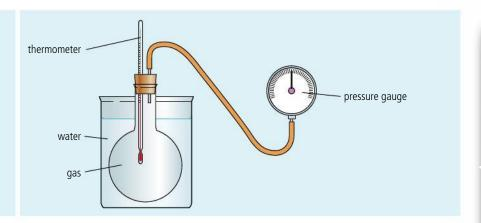
**Figure 3.48** Apparatus to measure *P* and *T*.
