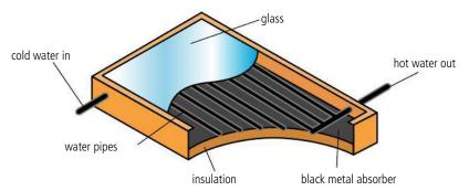
Solar heating panels can be used for central heating or for making water hot for household use. They are placed on the roofs of houses. Solar radiation enters the panel through the glass cover, is absorbed by a black metal plate which gets hot, and in turn makes the water hot by conduction. Water is continuously circulated so that, as the water gets hot, it flows out and more cold water flows in.
