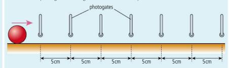
This is would be quite expensive so we compromise by using just two photogates and a motion that can be repeated. An example could be a ball moving along a horizontal section of track after it has rolled down an inclined plane. Provided the ball starts from the same point it should have the same velocity. So instead of using seven photogates we can use two, one is set at the start of the motion and the other is moved to different positions along the track as in Figure 2.7.
