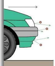
**Figure 3.15** The front of the car collides with air molecules.
