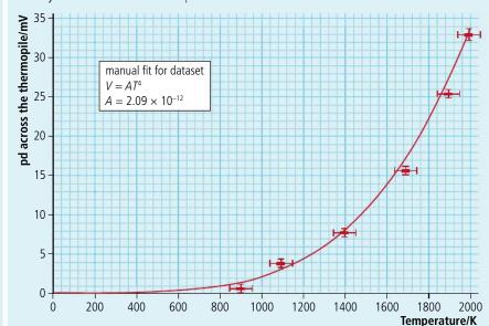
This is obviously not a straight line but the curve  $y = 2.09 \times 10^{-12} x^4$  is a good fit. Since the thermopile pd is proportional to the power absorbed per unit area, this shows that:
