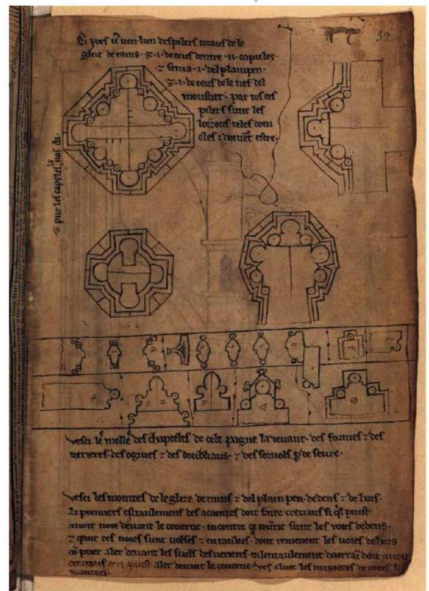
Templates in an architectural sketchbook by Villard de Honnecourt, held in the Bibliothèque Nationale de France in Paris.
