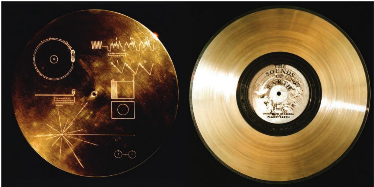
↑ Figure 3.2 The Golden Record, attached to each of the Voyager spacecraft, is a 12-inch gold-plated phonograph record, containing sound and images from Earth (right) and a cover (left) containing instructions about how to “play” the record and where it comes from
